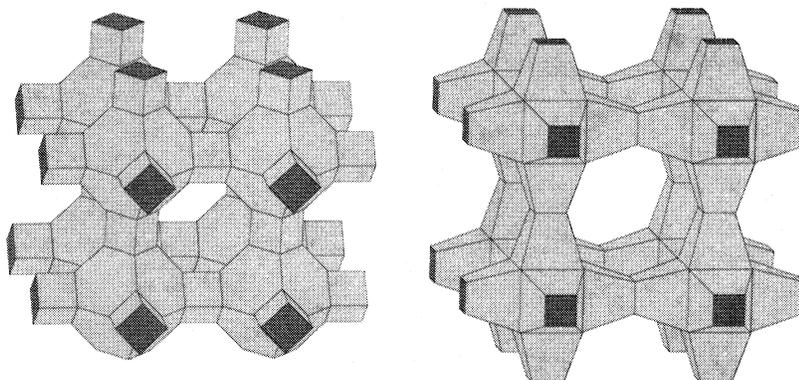
**Figure 2:**  $(4^26^2)$  In this example, which can be constructed from a space-filling arrangement of semi-regular polyhedra and cubes, space is not divided into congruent halves. The missing polyhedra are rhombi-truncated cuboctahedra. It is possible to construct a dual that has vertices at the centroids of the faces.
