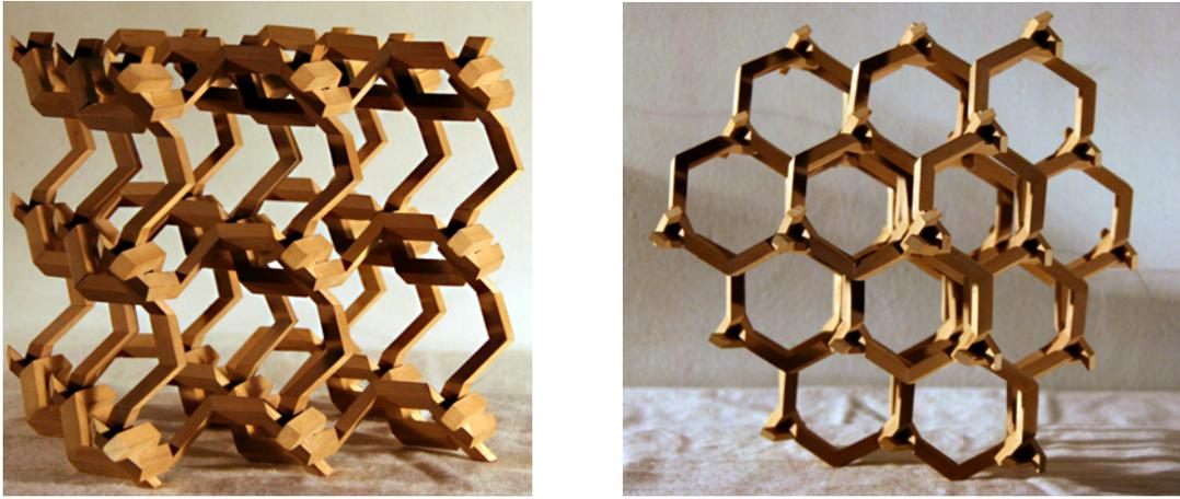
**Figure 12:** Space-spanning mesh from non-parallel zigzagzugs with rhombic cross section and skew miter joints (square cut faces), three strands link at each meeting point, each strand having its “own” axis direction (orthogonal)
