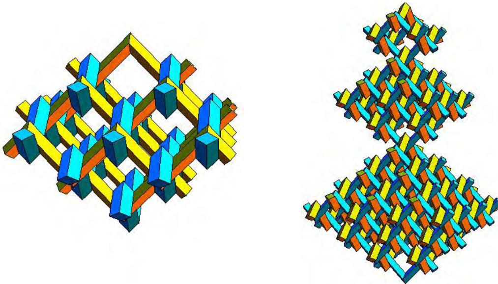
**Figure 3:** Single octahedron (left) and chain of hanging octahedrons (right) constructed from woven zigzags with a rhombic cross section
