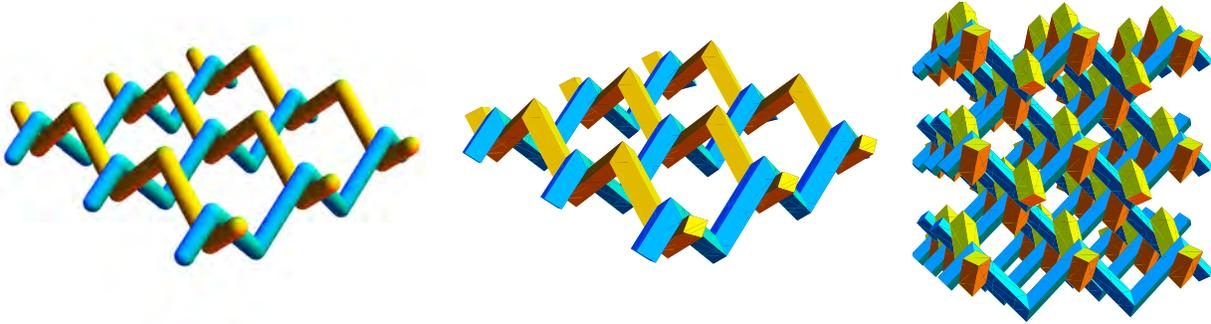
**Figure 2:** Space-spanning mesh constructed from orthogonally crossing zigzags; left: single layer using bent tubes; center: single layer using rhombic beams and miter joints; right: extension into 3D
