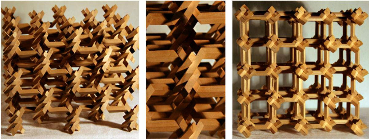
**Figure 11:** Space-spanning mesh from non-parallel zigzagzags with rhombic cross section and skew miter joints (square cut faces), four strands link at each meeting point, each strand having its “own” axis direction (main diagonals of the cube)
