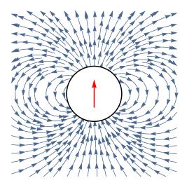
**Figure 9**: A horizontal slice of the external field of one magnet with moment  $\vec{m} = (0, 1)$ .
