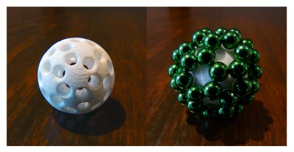
Figure 8: A 3D printed scaffold, and a buckyball of buckyballs arranged upon it.
