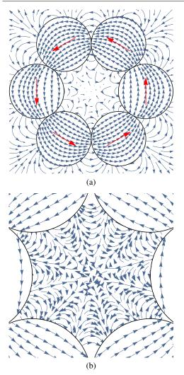
Figure 10: Magnetic field from a hexagonal loop on the plane of the loop. Inside each magnet, only the total of the contributions to the magnetic field from all other magnets is shown. Outside of the circles, the total contribution from all magnets is shown. Figure 10b shows a closeup view of the center of the loop.
