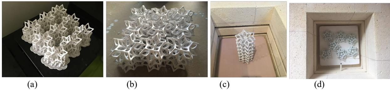
**Figure 4:** Ceramic fabrication process (a) a 3D printed formation showing the support system used to anchor the pieces while printing (b) a formation after cleaning the 3D printing supports, (c) A stack of pieces after first firing to burn the polymer matrix in the kiln, (d) the second firing to apply the glaze.
